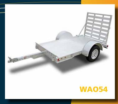
One couldn't ask for a more dependable sidekick than the WAO54 open ATV trailer. It's a compact design makes it easy to tow and it comes standard with a convenient folding ramp. The extruded aluminum floor and all LED lighting provide enhanced safety. In addition to hauling ATV's, the WAO54 is perfect for hauling motorcycles, riding lawn mowers and other equipment. Value comes in all sizes and the WAO54 packs a lot of utility in a small footprint.
