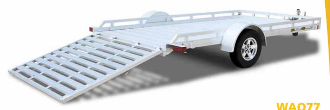
The Wells Cargo SilverSport model WAO77 is an all-aluminum trailer that's ideal for recreational ATV owners. It is available in 10', 12' or 14' lengths with a 6'6" width. The standard stake pockets (8 or 10) give you maximum cargo control flexibility. The WAO77 also features a standard ramp, slip resistant extruded aluminum floor, and all LED lighting for improved safety.
