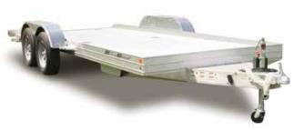
The open car trailer model WACO79 ranges in length from 14' to 24'. It has a width of 8' or 8'6" depending on the length of the trailer. The WACO79 rides on tandem Dexter Torflex® axles with EZ-Lube Hubs and Electric Brakes. It also features stainless steel swivel D-Rings, removable fenders and ramps (2) that store underneath the trailer. Ask about the Power Tilt option that eliminates the need for rear ramps.
